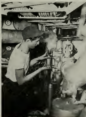
Midshipman R. Kuykendall overhauling valve chest on pump.
